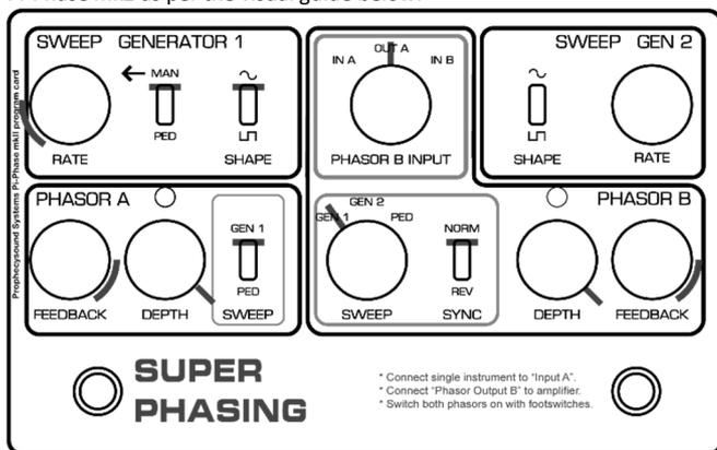
The signal from [PHASOR B OUTPUT] is processed by all 12-phase stages within your Pi-Phase mk2 for the deepest and most lush sound; note that both PHASOR A and PHASOR B are modulated by the same control signal, that being GEN 1. Experiment with different settings within this program, for example turning the [FEEDBACK] controls of both PHASOR A and PHASOR B down to minimum, or by adjusting the [DEPTH] controls for both sections for a more subtle effect.
