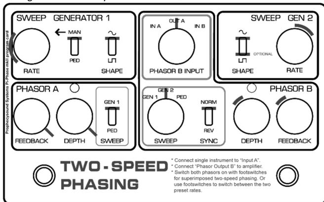
Using this setting you can switch PHASOR A and PHASOR B on or off to create a phased signal with two different modulation types layered, or with the audio processed by a single phase section.
